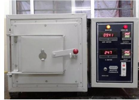
**Door:** Adequate Insulated Rectangular door made of thick SS sheet with counter balanced door opening arrangement is provided with a parallel swing a side opened. The door is fitted at the thick MS plate. The Door having centre hole with sliding window for viewing the furnace chamber while in operation.
